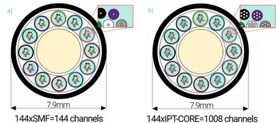
Fig. 1. a) Fiber optic cable with SMFs; b) Fiber optic cable with InPhoTech's MCF.
