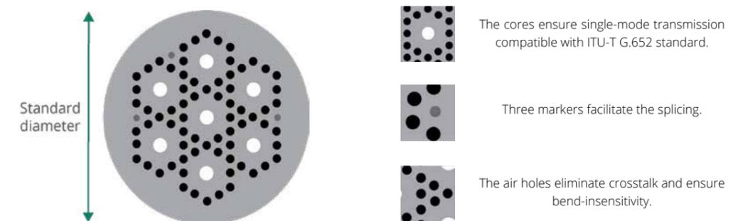
Fig. 5. InPhoTech's MCF structure with its characteristic elements.
