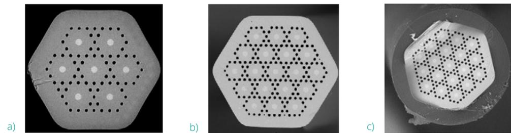
Fig. 7. Microscope images of the cross-section of a) 7-core fiber b) 19-core fiber c) 19-core fiber with coating.
