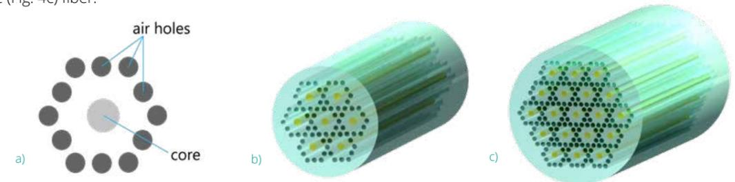
Fig. 4. a) MCF's basic cell; b) 7-core fiber design; c) 19-core fiber design.
